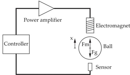
Figure 2: Arrangement of a magnetic bearing
