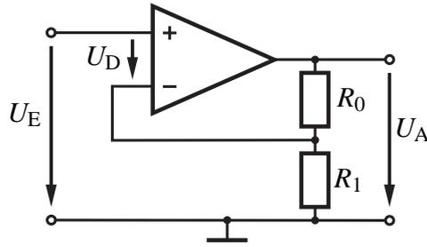
Figure 10: Non-inverting amplifier
