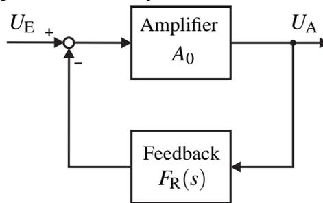
Figure 9: Basic principle of feedback
