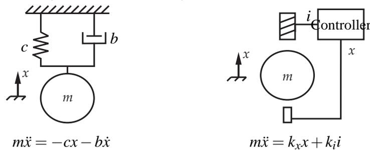
Figure 5: Comparison of physical equivalent circuit model and magnetic bearing
