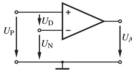
Figure 7: Open-loop operational amplifier
