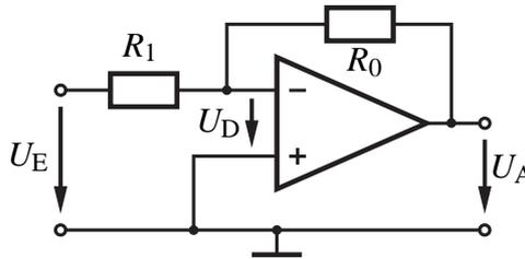
Figure 11: Inverting amplifier
