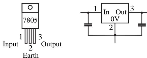
Figure 16: Pin numbering and simplified circuit diagram
