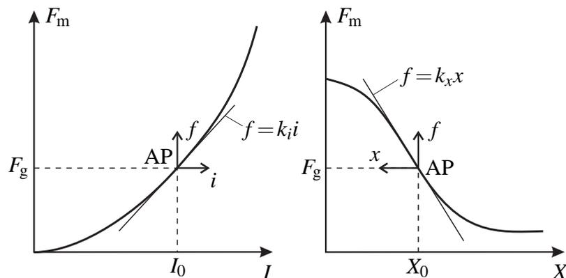
Figure 3: Magnetising curves of an electromagnet
