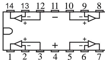
Figure 15: Op amp pin numbering
