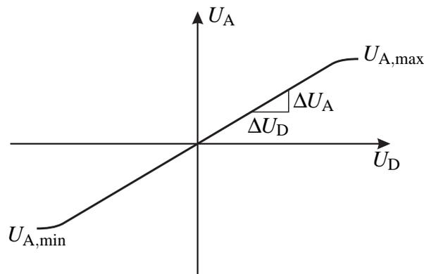
Figure 8: Curve of operational amplifier
