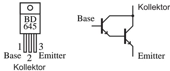
Figure 17: Darlington transistor BD645 with internal circuit diagram
