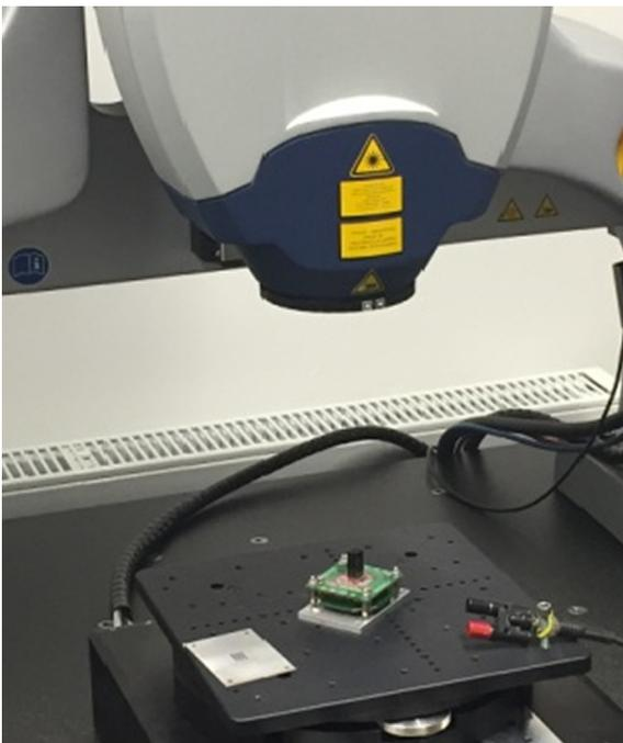
Fig. 3. MSA-100-3d-M Micro System Analyzer with a tactile display.
